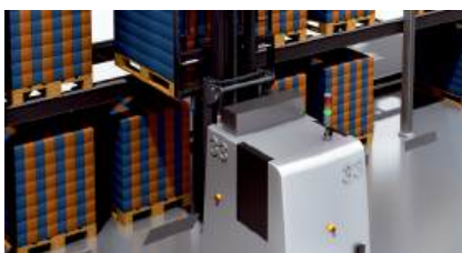
Empty bay detection with automated guided vehicles
